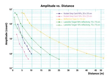
The chart above displays the detection amplitude of a 450 sensor for five reference objects (photography grey cards and reflective tape) of varying size and reflectivity.
